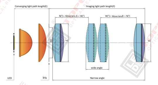
②As shown in the following diagram, the part of imaging lens set consists of three achromatic cemented lenses. We can divide these three lenses into two groups. From left to right, group 1 includes A and B, group 2 is C. This is a zoom system, it output wide beam when two lens groups are closing to each other, if the two lens groups move away from each other, the output beam will be narrow-angle.
